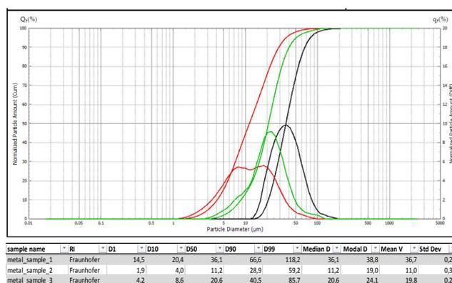
Figure 2: different metal powders measured with our SALD-2300 with MS-23
